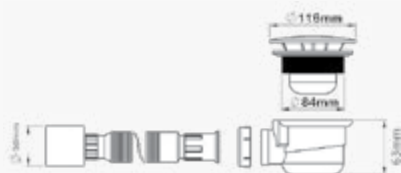
5206836100197 Sifone valvola ABS, Φ90. Valve siphon ABS, Φ90. Siphon vanne ABS, Φ90. Βαλβίδα ABS, Φ90.
